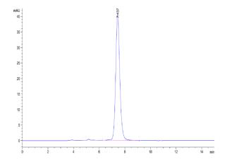
The purity of Mouse PD-1 is greater than 95% as determined by SEC-HPLC.
